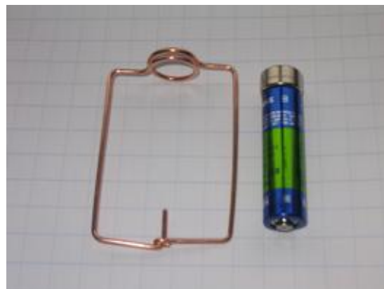
The finished loop and battery with the magnet
