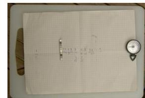
As a second step, I did the same with nine magnets, then with eight and so on, until only a single magnet turned the compass by 90 degrees.
