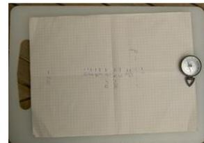
Next, I stacked the 10 cube magnets and oriented them on the sheet in such a way that they would affect the compass needle. I then tested at which magnet distance the compass needle would turn 90 degrees towards the magnets. At that point, I made a mark on the paper and also noted the number of magnets.
