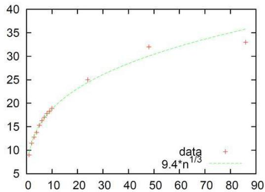
If you plot the mass of the magnets (x-axis) against the distance in centimetres (y-axis), it is consistent with our  $1/R^3$  law. The cube magnets weigh 1 gram, the large magnets 24 and 48 grams, respectively. The data is not entirely accurate because I didn't measure as precisely off the paper. However, the trend is consistent.
