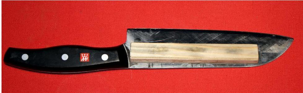
When sharpening the kitchen knives it's important to keep a constant angle of about 15 degrees between knife and sharpening block to get a good result. A ledge that helps to maintain the correct angle is easily made.
