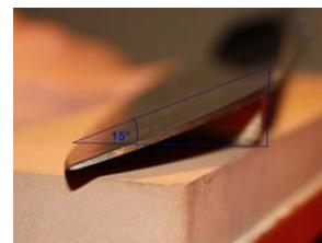
When sharpening you have to make sure that the ledge lies straight - then you automatically maintain a constant angle (15 degrees with the above measurements).
