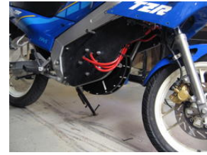
The Yamaha after the modification with a functional electric motor!
