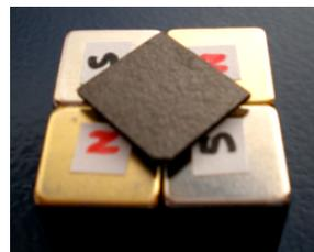
Remove the small stickers and place the graphite disc carefully over the four magnets. You will observe that the graphite disc levitates above the four magnets endlessly (yes, for minutes, hours, days, weeks, months...) The height of the levitation is approximately 2-3 millimeters and clearly visible. We can even push the tiny disc down with a finger, let it go and observe how it climbs again to levitate in the same place as before.
