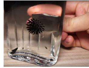
Why straight walls on the glass container? Due to light refraction it is hard to observe ferrofluid in bent bottles.
