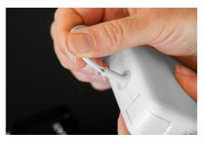
insulating and sealing effect. And since Sugru remains pliable when dry, the cable stays flexible.
